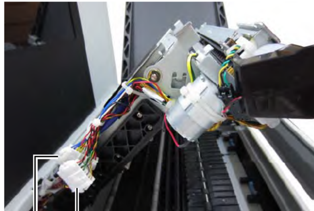
Figure 6 Connectors and cables on left side of clamshell
